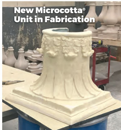
3-D Printed Replica (for mold)
