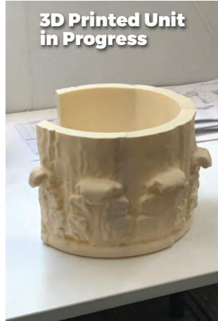
New Microcotta® Unit in Fabrication
